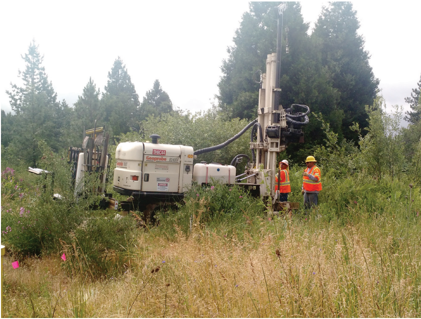
Soil extraction for testing of the Roseburg property in Mount Shasta, California. The testing is part of an Environmental Protection Agency Brownfields Grant. (Source: © 2016 Juliana Lucchesi (CC BY-NC 4.0), from the American Planning Association's Image Library.)
